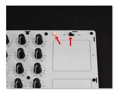
The device can now be powered on by turning the Power Switch to the ON position. This will be indicated by the red light as shown in the picture.
