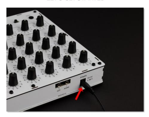
Start by connecting the jack end of the adaptor to the socket on the rear of the device marked "POWER 12V DC" as shown in the picture above.
